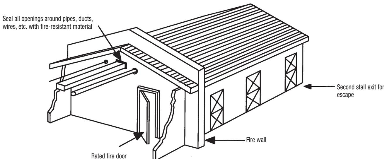
**Figure 4. Fire curtain to delay and limit the horizontal spread of heat, smoke, and flame.**
